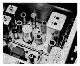
socket on the plate and fabricate a small brass shield about 5/8 inch (1.6cm) high. This shield is placed across the tube socket between pins 3-4 and 8-9 and soldered in place (see mechanical filter sockets A, B and C for reference). Ground all unused socket pins.
